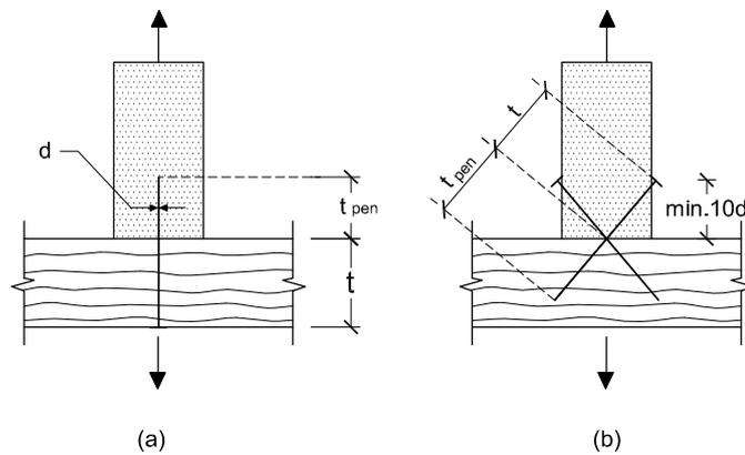
Figura 8.8, Clavado perpendicular (a) y oblicuo (b)
